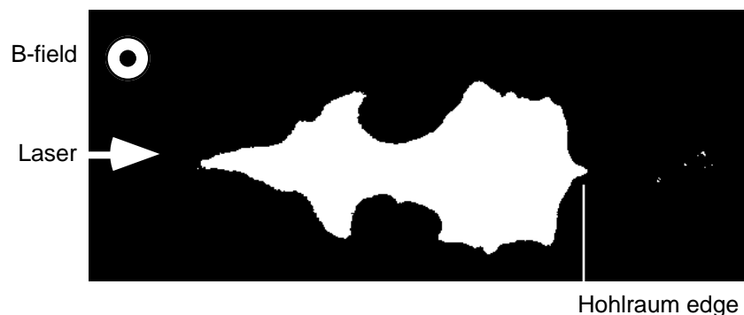
Figure VII-4. Optical image of a plasma streaming into a magnetic field. The plasma jet is emerging from a hohlraum on the right into a B-field that is coming out of the plane of the figure. The image was taken at 850 ns after the laser pulse started, using an ultrafast optical framing camera with 2-ns time resolution. Note the dramatic vortex structure.
